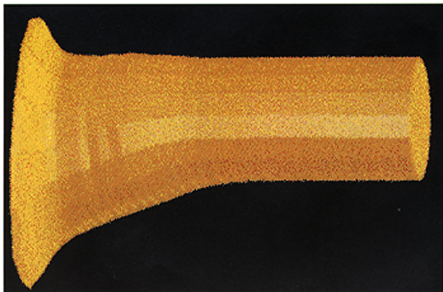
Plate 2. Deformed shape of the bar for the oblique impact at 80 \mu seconds
